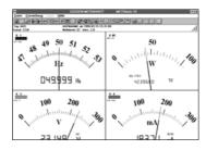
Transmitted measurement values from a maximum of four freely selectable channels are displayed at the monitor in the online mode either in digital format with additional analog scale, or as an analog pointer instrument with additional digital display.
